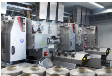
Caption: The yarn was produced on a Neumag S8 BCF system with a BICO spinning beam.
