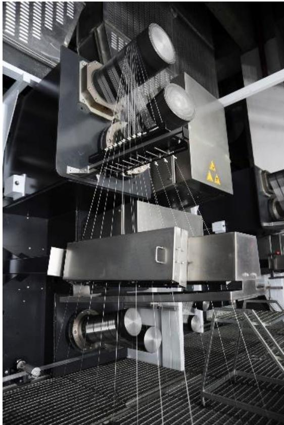
Airbags, safety belts, tire cord, geotextiles, safety ropes, conveyor belts – Oerlikon Barmag industrial yarn systems manufacture filament yarns for the most diverse applications.
