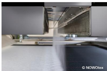
Caption: The Oerlikon Nonwoven meltblown spinning process excels as a result of homogeneous nonwoven properties and running meter weights.
